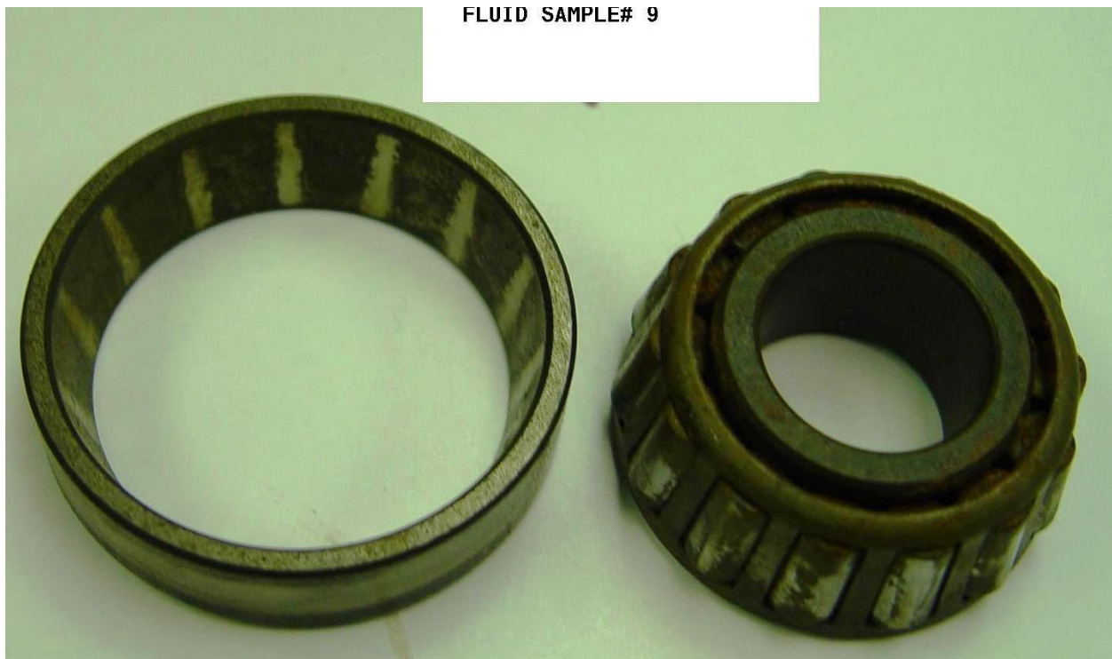
Figure 3. Bearing after test with Krytox FG-50
