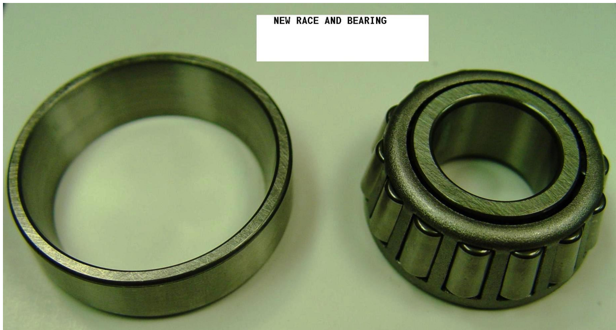
Figure 1. New bearing, before modified ASTM D1743 testing
